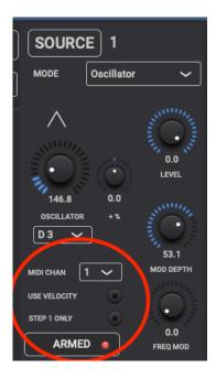
For any DAW/Host configuration you first have to enable the midi in for the Sequencer Oscillator Source :
