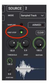
When playing live another setting you may want to use is the "Sustain" (in seconds!). When the value is not zero or 100s, the sampled audio will decrease in level to reach zero after the time set. You then have to re-sample to make the audio active again (or set the Sustain to zero or 100).
