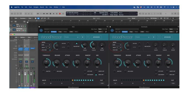
Linking is different from side-chaining : in side-chain compression the GR is ONLY calculated by the side chain audio and not by the track audio on which the compressor is inserted.
