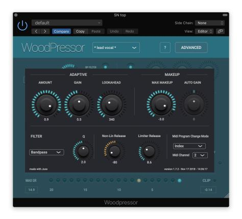
The Advanced panel can be made visible by pressing the "Advanced" button.
